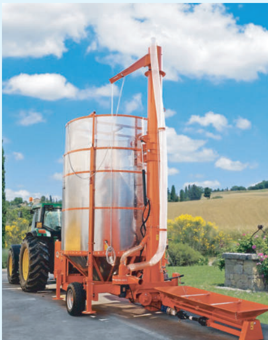
Mobile Drier Using PTO on 70Hp Tractor
