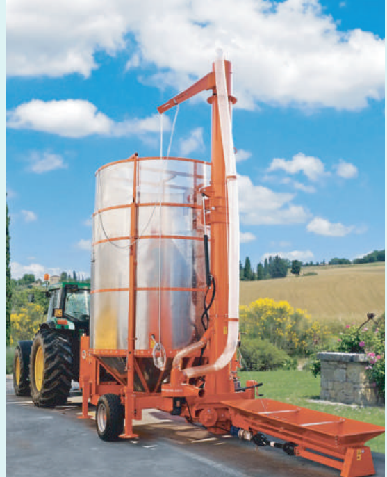
Mobile Drier Using PTO on 70Hp Tractor
